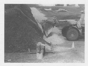
The Com-Til Facility in Columbus, Ohio, composts biosolids. Wood chips, recycled compost and sawdust are added as bulking agents. The facility handles 50,000 wet tons of biosolids each year—25 dry tons per day. One eighth of the volume produced is sold as bagged compost and the remainder as bulk compost. The facility features an open concrete pad. Compost is piled 10- to 12-feet high on perforated plastic tile to achieve updraft aeration.
